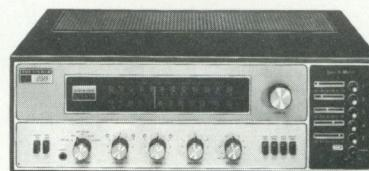
**Model 250T** 100-Watt AM-FM Stereo Receiver with two separate modes of tuning: Push-Button and Conventional Flywheel tuning. Enormous reserve power and performance surpassing anything in its price class. Price . . . . . \$569.95
