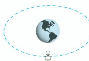
To be geostationary, a satellite's orbital distance must be about 36,000 km (22,300 miles) above the earth's surface and the orbital speed must be a critical 11,062 km per hour (6,875 miles per hour). The moon at 388,000 km (240,000 miles) from earth requires 28 days to orbit the earth at a speed of 3,540 km per hour (2,200 miles per hour). A satellite at 161 km (100 miles) from earth would complete an orbit in one-and-a-half hours at a speed of 27,400 km per hour (17,000 miles per hour).
