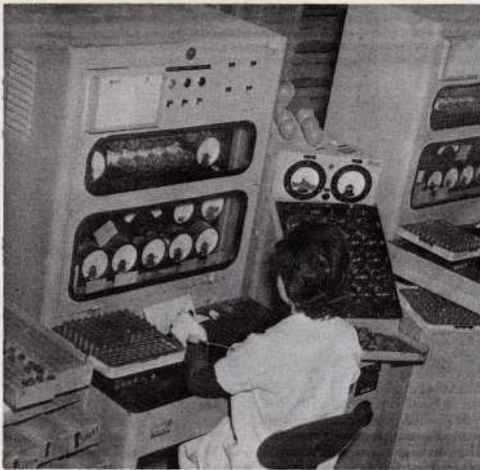
One of Cowansville's skillful tube testers sitting in front of a testing console. Each tube is checked for shorts in continuity, gas, light current and emission. The examination in this photo are being done by Therese Perrault.
