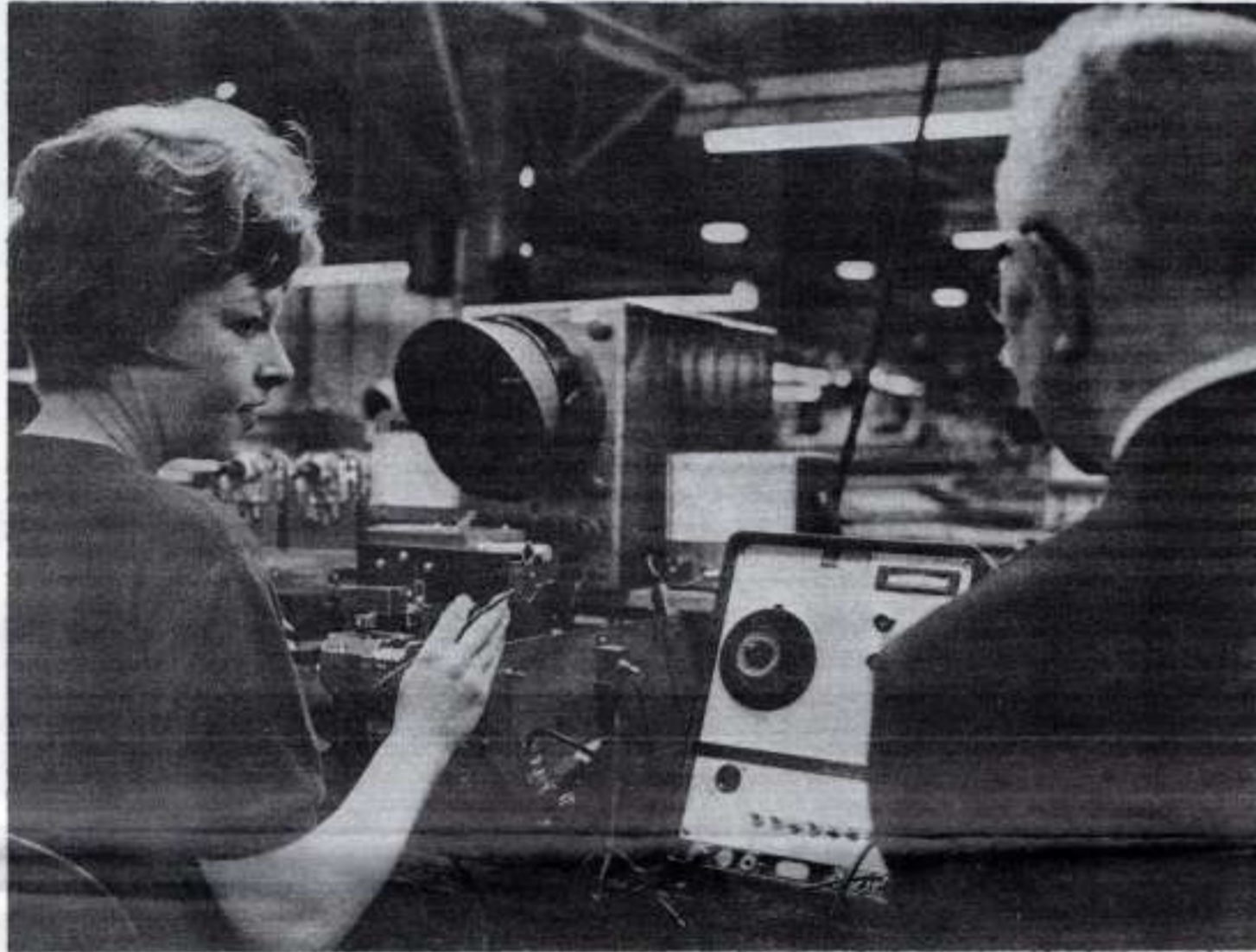
A visitor to the Renfrew Plant watches Beverley Utronki performing the alignment and final test on a very high frequency tuner. (Photo - Renfrew Advance)
